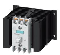
Solid-state contactor 3-phase 3RF2 AC 51 / 50 A / 40  $^\circ$ C 48-600 V / 4-30 V DC 2-phase controlled Ring cable connection Blocking voltage 1200 V
