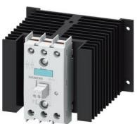
Solid-state contactor 3-phase 3RF2 AC 51 / 50 A / 40  $^\circ\rm{C}$  48-600 V / 110 V AC 2-phase controlled screw terminal Blocking voltage 1200 V
