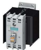
Solid-state contactor 3-phase 3RF2 AC 51 / 20 A / 40  $^\circ$ C 48-600 V / 4-30 V DC 3-phase controlled Spring-type terminal Blocking voltage 1200 V
