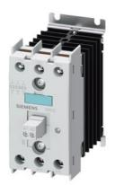
Solid-state contactor 3-phase 3RF2 AC 51 / 10 A / 40  $^{\circ}\text{C}$  48-600 V / 4-30 V DC 3-phase controlled screw terminal Blocking voltage 1200 V
