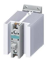
Solid-state contactor 1-phase 3RF2 AC 51 / 40 A / 40  $^{\circ}\text{C}$  24-230 V / 110-230 V AC Ring cable connection
