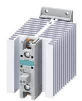
Solid-state contactor 1-phase 3RF2 AC 51 / 40 A / 40  $^{\circ}\text{C}$  48-600 V / 24 V DC Ring cable connection
