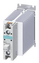
Solid-state contactor 1-phase 3RF2 AC 51 / 30 A / 40  $^{\circ}\text{C}$  24-230 V / 110-230 V AC Ring cable connection
