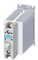
Solid-state contactor 1-phase 3RF2 AC 51 / 30 A / 40  $^{\circ}\text{C}$  24-230 V / 24 V DC Ring cable connection
