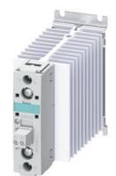
Solid-state contactor 1-phase 3RF2 AC 15 / 15 A / 40  $^\circ\text{C}$  24-230 V / 24 V DC Instantaneous switching
