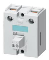
Semiconductor relay, 1-phase 3RF2 Overall width 45 mm, 30 A 48-600 V / 24 V DC screw terminal
