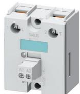
Semiconductor relay, 1-phase 3RF2 Width 45 mm, 20 A 48-600 V / 4-30 V DC screw terminal Blocking voltage 1200 V
