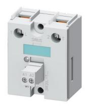
Semiconductor relay, 1-phase 3RF2 Width 45 mm, 20 A 24-230 V / 4-30 V DC screw terminal
