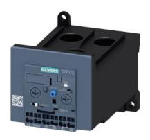
Overload relay 32...115 A Electronic For motor protection Size S3, Class 5E...30E Stand-alone installation Main circuit: Straight-through transformer Auxiliary circuit: Spring-type terminal Manual-Automatic-Reset
