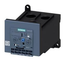
Overload relay 12.5...50 A Electronic For motor protection Size S3, Class 5E...30E Stand-alone installation Main circuit: Straight-through transformer Auxiliary circuit: Spring-type terminal Manual-Automatic-Reset
