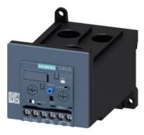
Overload relay 12.5...50 A Electronic For motor protection Size S3, Class 5E...30E Stand-alone installation Main circuit: Straight-through transformer Auxiliary circuit: Screw Manual-Automatic-Reset
