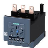
Overload relay 12.5...50 A Electronic For motor protection Size S3, Class 5E...30E Contactor mounting Main circuit: Screw Auxiliary circuit: Screw Manual-Automatic-Reset
