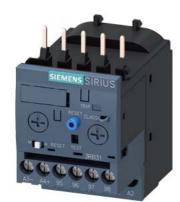
Overload relay 4...16 A Electronic For motor protection Size S00, Class 5...30 Contactor mounting Main circuit: Screw Auxiliary circuit: Screw Manual-Automatic-Reset Internal ground fault detection
