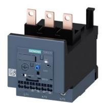
Overload relay 32...115 A Electronic For motor protection Size S3, Class 20E Contactor mounting Main circuit: Screw Auxiliary circuit: Spring-type terminal Manual-Automatic-Reset
