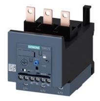
Overload relay 32...115 A Electronic For motor protection Size S3, Class 20E Contactor mounting Main circuit: Screw Auxiliary circuit: Screw Manual-Automatic-Reset
