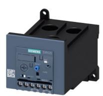
Overload relay 12.5...50 A Electronic For motor protection Size S3, Class 20E Stand-alone installation Main circuit: Straight-through transformer Auxiliary circuit: Screw Manual-Automatic-Reset
