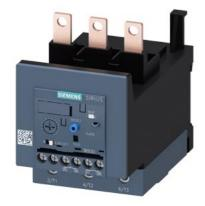
Overload relay 12.5...50 A Electronic For motor protection Size S3, Class 20E Contactor mounting Main circuit: Screw Auxiliary circuit: Screw Manual-Automatic-Reset
