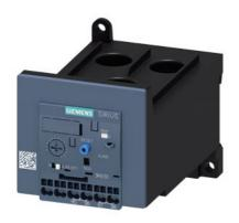
Overload relay 32...115 A Electronic For motor protection Size S3, Class 10E Stand-alone installation Main circuit: Straight-through transformer Auxiliary circuit: Spring-type terminal Manual-Automatic-Reset
