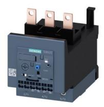
Overload relay 32...115 A Electronic For motor protection Size S3, Class 10E Contactor mounting Main circuit: Screw Auxiliary circuit: Spring-type terminal Manual-Automatic-Reset
