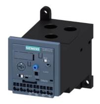
Overload relay 12.5...50 A Electronic For motor protection Size S2, Class 20E Stand-alone installation Main circuit: Straight-through transformer Auxiliary circuit: Spring-type terminal Manual-Automatic-Reset
