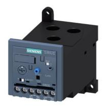
Overload relay 12.5...50 A Electronic For motor protection Size S2, Class 20E Stand-alone installation Main circuit: Straight-through transformer Auxiliary circuit: Screw Manual-Automatic-Reset
