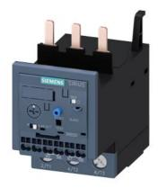
Overload relay 12.5...50 A Electronic For motor protection Size S2, Class 20E Contactor mounting Main circuit: Screw Auxiliary circuit: Spring-type terminal Manual-Automatic-Reset
