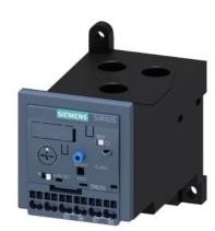
Overload relay 20...80 A Electronic For motor protection Size S2, Class 10E Standalone installation Main circuit: Straight-through transformer Auxiliary circuit: Springtype terminal Manual-Automatic-Reset
