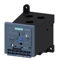
Overload relay 12.5...50 A Electronic For motor protection Size S2, Class 10E Stand-alone installation Main circuit: Straight-through transformer Auxiliary circuit: Spring-type terminal Manual-Automatic-Reset
