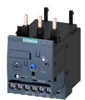
Overload relay 10...40 A Electronic For motor protection Size S0, Class 20 Contactor mounting Main circuit: Screw Auxiliary circuit: Screw Manual-Automatic-Reset
