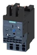
Overload relay 3...12 A Electronic For motor protection Size S0, Class 20 Contactor mounting Main circuit: Spring-type terminal Auxiliary circuit: Spring-type terminal Manual-Automatic-Reset
