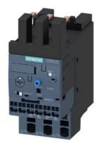
Overload relay 1...4 A Electronic For motor protection Size S0, Class 20 Contactor mounting Main circuit: Spring-type terminal Auxiliary circuit: Spring-type terminal Manual-Automatic-Reset
