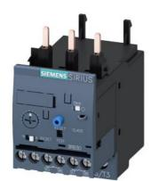
Overload relay 0.32...1.25 A Electronic For motor protection Size S0, Class 20E Contactor mounting Main circuit: Screw Auxiliary circuit: Screw Manual-Automatic-Reset
