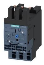
Overload relay 1...4 A Electronic For motor protection Size S0, Class 10E Contactor mounting Main circuit: Spring-type terminal Auxiliary circuit: Spring-type terminal Manual-Automatic-Reset
