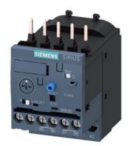
Overload relay 3...12 A Electronic For motor protection Size S00, Class 20E Contactor mounting Main circuit: Screw Auxiliary circuit: Screw Manual-Automatic-Reset
