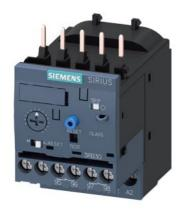
Overload relay 0.1...0.4 A Electronic For motor protection Size S00, Class 20E Contactor mounting Main circuit: Screw Auxiliary circuit: Screw Manual-Automatic-Reset
