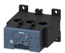
Overload relay 50...200 A for motor protection Size S6, CLASS 5...30E Contactor mounting/stand-alone installation Main circuit: straight-through transformer Auxiliary circuit: Spring-type terminal Manual-Automatic-Reset Internal ground fault detection
