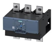
Overload relay 160...630 A for motor protection Size S10/S12, Class 20E Contactor mounting/stand-alone installation Main circuit: busbar connection Auxiliary circuit: Spring-type terminal Manual-Automatic-Reset
