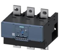
Overload relay 160...630 A for motor protection Size S10/S12, Class 20E Contactor mounting/stand-alone installation Main circuit: busbar connection Auxiliary circuit: Screw terminal Manual-Automatic-Reset
