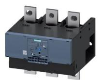
Overload relay 160...630 A for motor protection Size S10/S12, Class 10E Contactor mounting/stand-alone installation Main circuit: busbar connection Auxiliary circuit: Spring-type terminal Manual-Automatic-Reset
