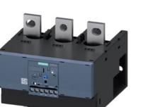
Overload relay 160...630 A for motor protection Size S10/S12, Class 10E Contactor mounting/stand-alone installation Main circuit: busbar connection Auxiliary circuit: Screw terminal Manual-Automatic-Reset
