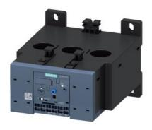
Overload relay 50...200 A for motor protection Size S6, Class 20E Contactor mounting/stand-alone installation Main circuit: straight-through transformer Auxiliary circuit: Spring-type terminal Manual-Automatic-Reset
