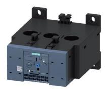
Overload relay 50...200 A for motor protection Size S6, Class 10E Contactor mounting/stand-alone installation Main circuit: straight-through transformer Auxiliary circuit: Spring-type terminal Manual-Automatic-Reset
