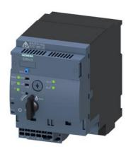
SIRIUS Compact load feeder Reversing starter for IO-Link 690 V 24 V DC 0.32...1.25 A IP20 Connection main circuit: plug-in, without terminals Connection control circuit: Spring-type terminal
