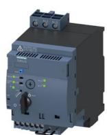
SIRIUS Compact load feeder Reversing starter for IO-Link 690 V 24 V DC 0.1...0.4 A IP20 Connection main circuit: Screw terminal Connection control circuit: screw terminal
