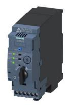
SIRIUS Compact load feeder DOL starter for IO-Link 690 V 24 V DC 1...4 A IP20 Connection main circuit: plug-in, without terminals Connection control circuit: screw terminal
