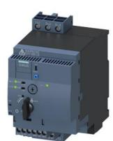
SIRIUS Compact load feeder Reversing starter 690 V 24 V AC/DC 50...60 Hz 3...12 A IP20 Connection main circuit: Screw terminal Connection control circuit: screw terminal
