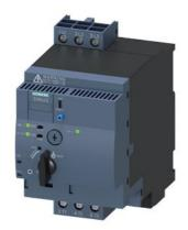
SIRIUS Compact load feeder Reversing starter 690 V 24 V AC/DC 50...60 Hz 1...4 A IP20 Connection main circuit: Screw terminal Connection control circuit: plug-in, without terminals
