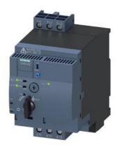
SIRIUS Compact load feeder Reversing starter 690 V 24 V AC/DC 50...60 Hz 0.1...0.4 A IP20 Connection main circuit: Screw terminal Connection control circuit: plug-in, without terminals
