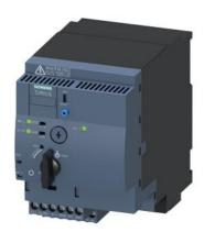
SIRIUS Compact load feeder Reversing starter 690 V 24 V AC/DC 50...60 Hz 0.1...0.4 A IP20 Connection main circuit: plug-in, without terminals Connection control circuit: screw terminal
