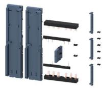
Wiring kit electrical and mechanical for complete load feeders fuseless, Size S3 for standard mounting rail mounting, consists of wiring module, busbar adapter and side modules
